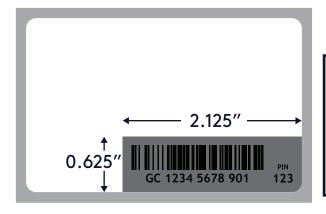
Note: leave 2.125" x 0.625" blank for barcode. Barcode can be placed anywhere.
